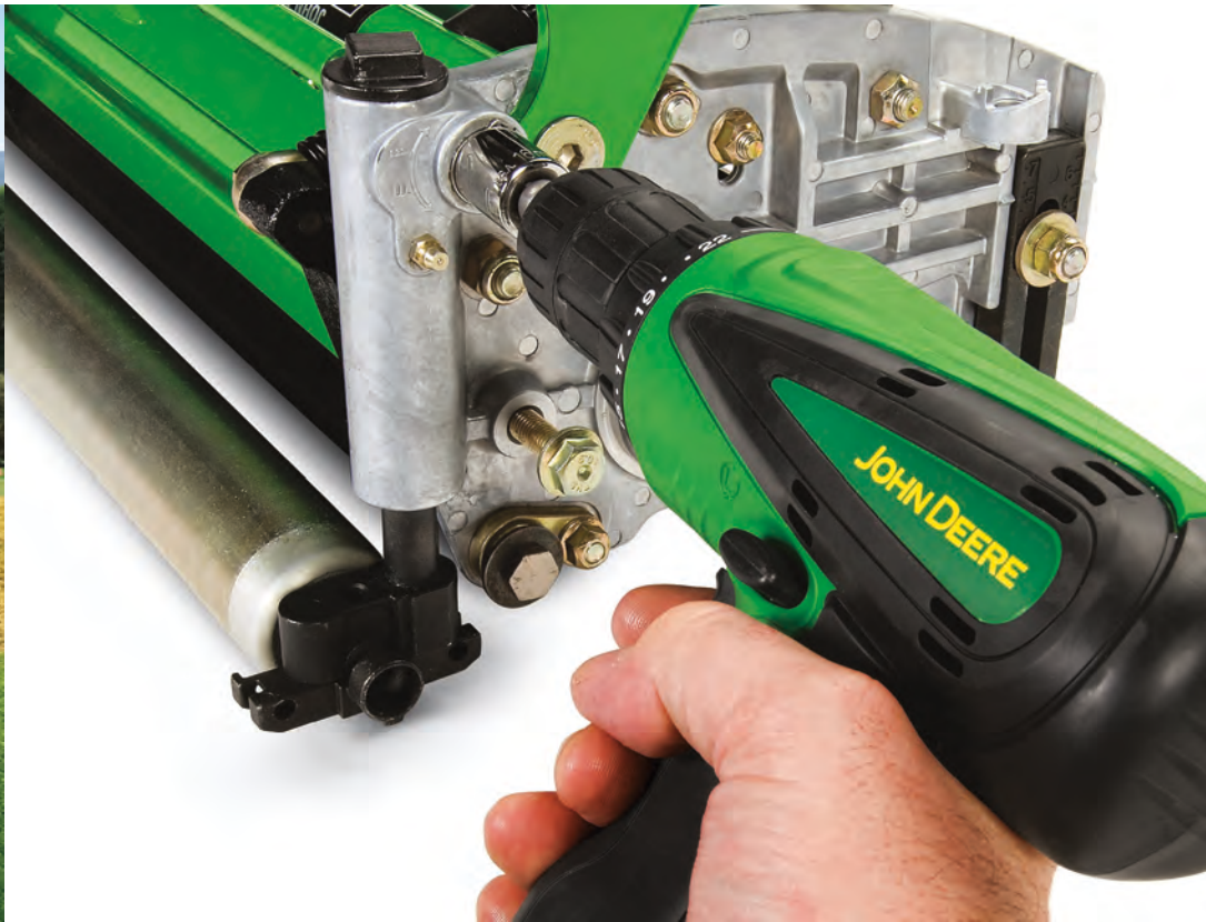
Rear roller power brush Prevents accumulation of grass clippings and other debris on the rear roller.
