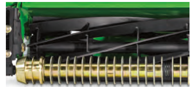
Rollers A full selection of spiral-grooved, continuous-grooved, and solid options.
